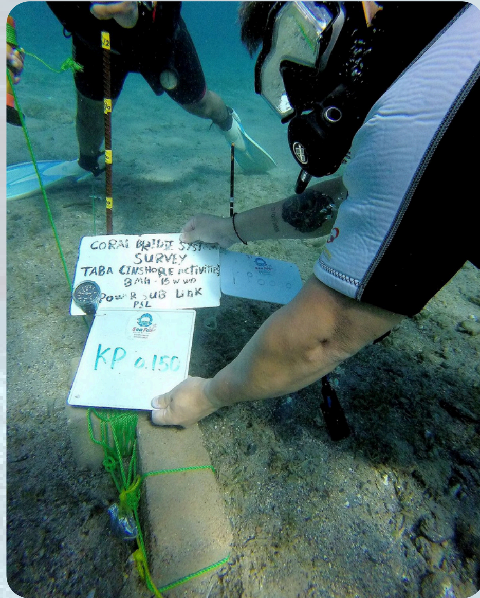
Seabed survey before Laying a cable for Telecom Egypt in Taba
